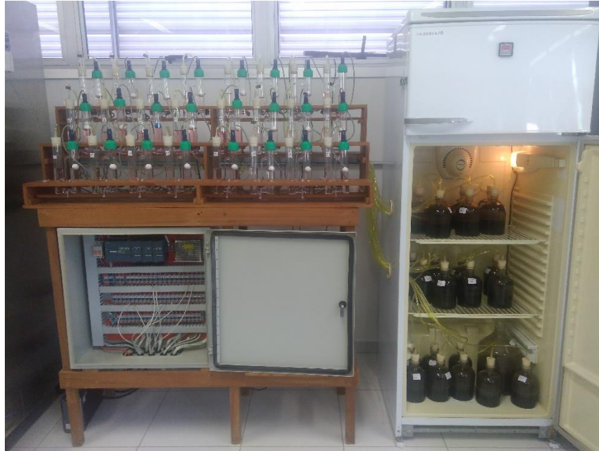
Fig. 2 Automated System for Biogas Measurement – SAMB
